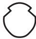
Grooved Trolley Wire Specification : ASTM B47 Copper Alloy UNS NO. C10700 (Silver Bearing)
