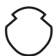
Grooved Trolley Wire Specification : ASTM B9 Copper Alloy UNS NO. C16200 (Alloy 80)
