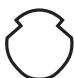
Grooved Trolley Wire Specification : ASTM B9 Copper Alloy UNS NO. C16500 (Alloy 55)
